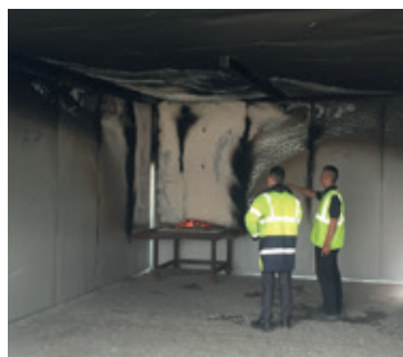
Inspection of protective char formation after test
