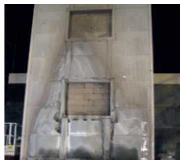
Façade after test demonstrating minimal fire spread attributable to the cladding
