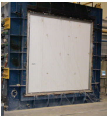
Vertical walls (3m x 3m furnace)
