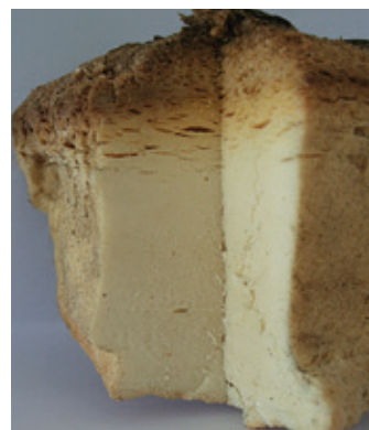
C: Temporary roof covering over hole in roof. D: PIR core showing delaminated lower surface and extent of through-thickness charring. E: Cut edge of lower steel skin of sandwich panel.
