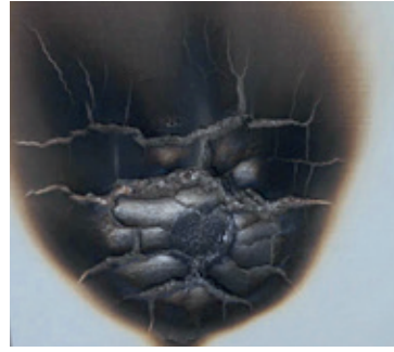
End of test showing localised char formation with no evidence of fire spread
