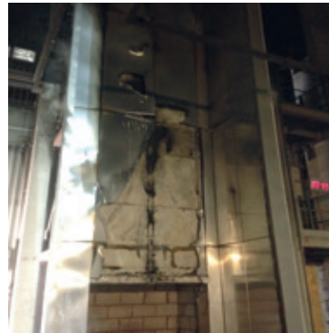
End of test showing aluminium cassette melted away to expose underlying Kingspan BENCHMARK Karrier panel in place
