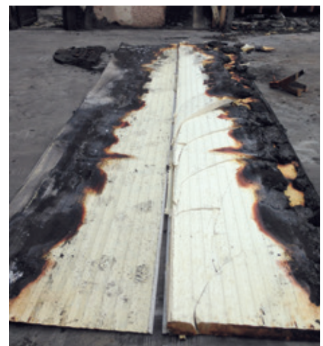
Panel at junction with steel stripped off demonstrating charring of PIR core but no evidence of fire spread.
