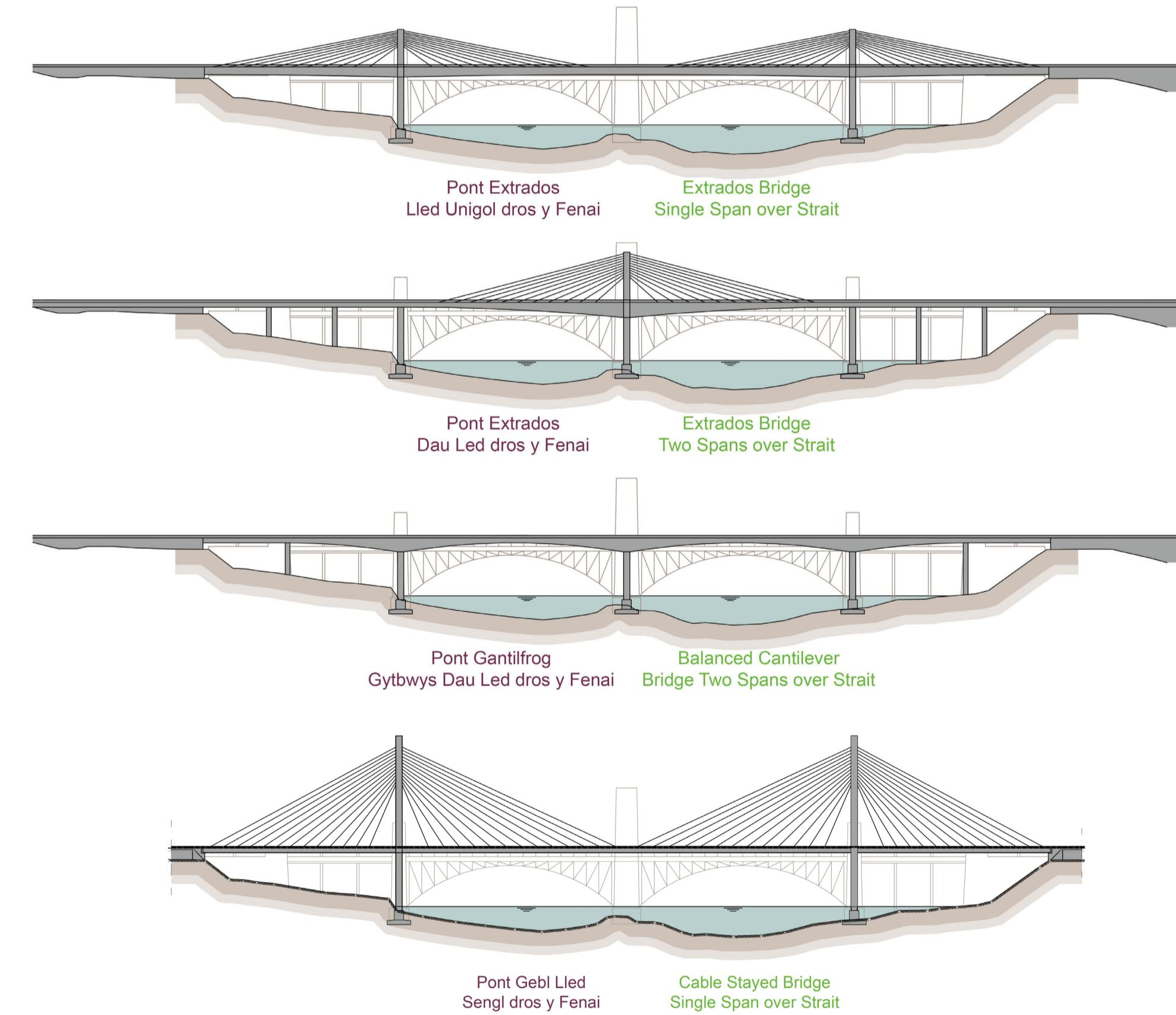
The following types of bridge construction are currently being considered. A preferred option will be identified as part of the current stage of work.
