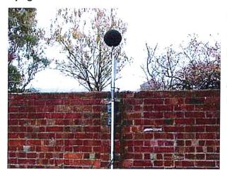
The microphone and windshield will be attached to a metal pole approximately 1.5 m to 4 m in length. The pole will then be secured to a solid upright structure, using a combination of cable ties and gaffer tape. Alternatively, the pole will extend directly from the environmental case.
