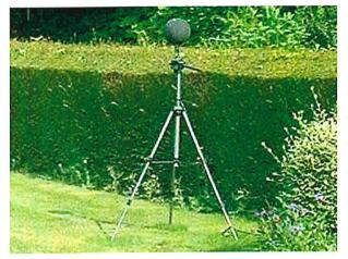
The tripod is a standard camera type tripod, which stands approximately 1.5 m tall. The tripod will be left freestanding in locations where it is unlikely to fall over and will not constitute a trip hazard. The feet of the tripod will be pegged into soft ground, the tripod will be counter weighted, or the tripod will be attached to a solid structure using cable ties or gaffer tape.
