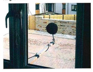
The sound level meter is located internally with the microphone cable running through the window to the microphone. The hinged frame is secured against the external sill, within the window aperture, and tied off to the window handle or suitable alternative internal point.
