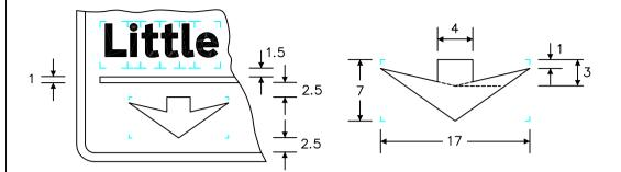
This dimension is reduced to 2.5sw when a junction name panel or grey backing board is provided.
