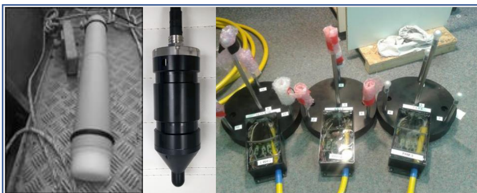
Ffigur 5. Enghreifftiau o offer hydrophone, C-POD (chwith), SoundTrap (canol, o Copping et al., 2020) a chlystwr hydrophone wedi'i adeiladu'n arbennig (dde, llun o Hastie et al., 2018).
