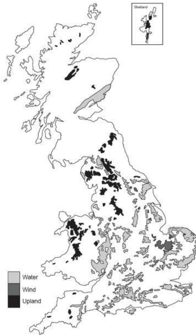
Figure 26. Areas of soil erosion risk in England, Wales and Scotland, based on land use, soil type and landform (i.e. slope). N.B. Upland includes both water and wind erosion. Source Defra SP08007 originally from Boardman and Evans, 2006.
