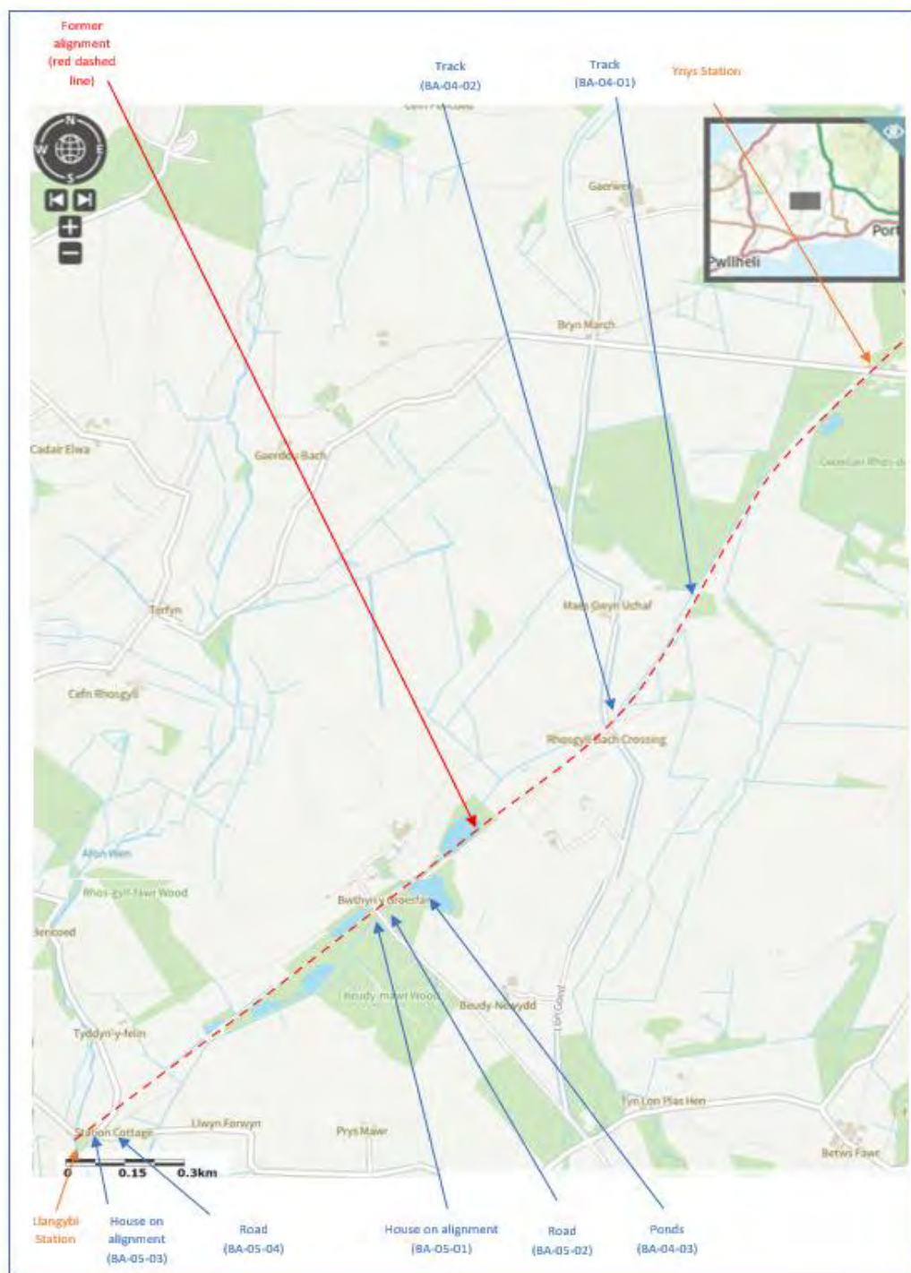
Figure 11-17 – Overview of Ynys Station to Llangybi Station showing obstructions along the route
