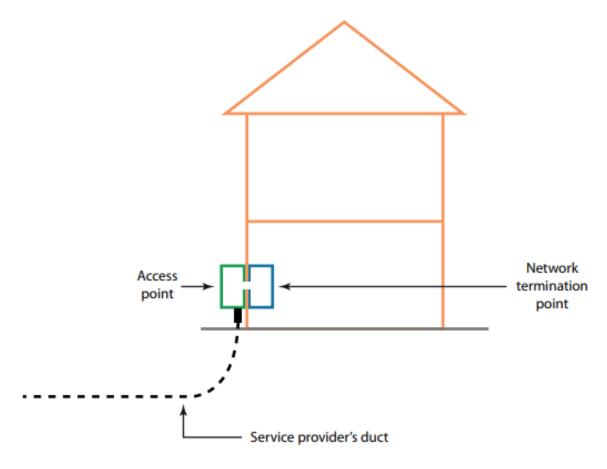
**Note:** The diagram shows future connectivity by underground ducts for network cables outside the building. However, it should be noted that alternative forms of connectivity may be used.
