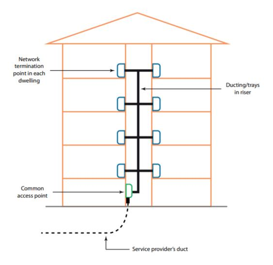
**Note:** The diagram shows future connectivity by underground ducts for network cables outside the building. However, it should be noted that alternative forms of connectivity may be used.
