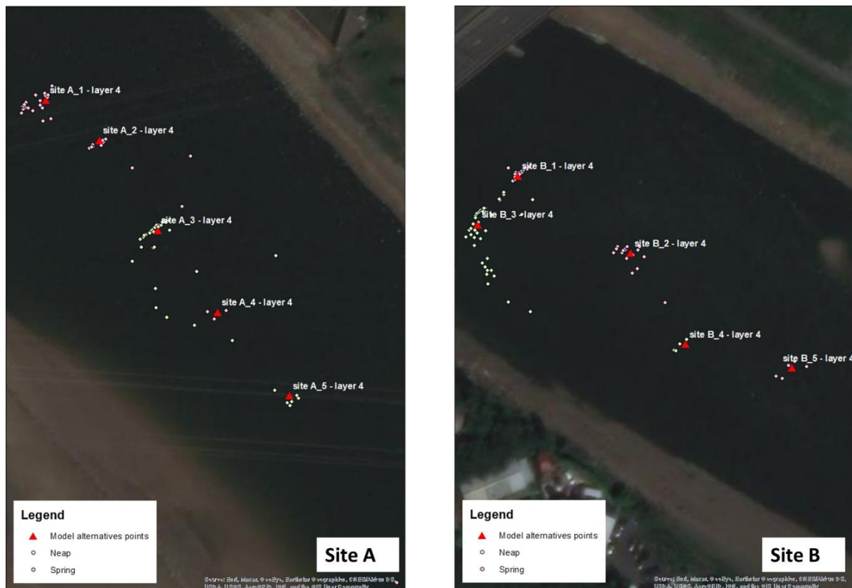
Figure 1-33 Movement of the boat during spring (pink points) and neap (green point) surveys at sites A and B. The red triangles show the additional current extraction locations selected to capture the boat mobility during the model calibration.
