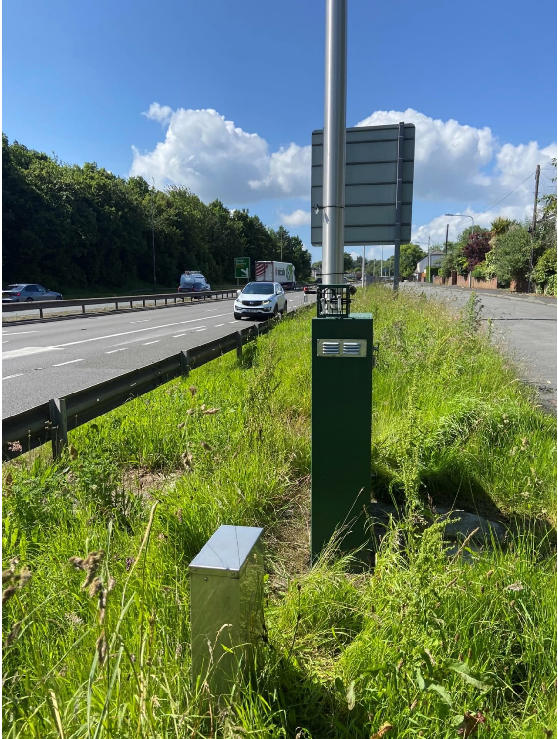
Figure C-1 Photo of diffusion tubes installed at Site D1
