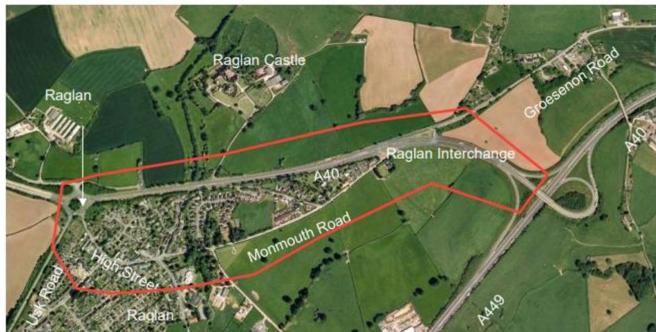
Substandard weaving distances between interchange and junctions.
