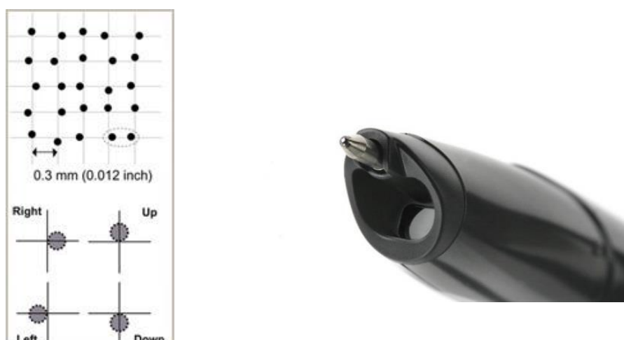
Figure 2: Digital pen and Anoto pattern
